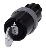
key-operated switch Siemens, 22 mm, round, plastic with metal front ring, lock number SSG10, with 2 keys, 3 switch positions I>O<II, momentary contact on the left, latching on the right, actuating angle  $2x45^\circ$ , 10:30h/12h/13:30h, key removal II, with laser labeling, upper case and lower case, always upper case at beginning of line
