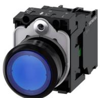
Illuminated pushbutton, 22 mm, round, plastic, blue, pushbutton, flat, momentary contact type, with holder, 1 NO, LED module with integrated LED 24 V AC/DC, screw terminal
