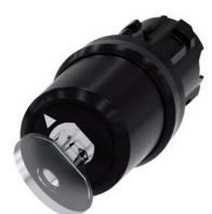
keyswitch BKS, 22 mm, round, plastic, special lock, with 2 keys, 2 switch positions O<I, momentary contact type, actuating angle 45°, 10:30h/12h, key removal O, note: for the BKS locking systems E1 - E25 supplied without key
