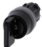
Key-operated switch O.M.R, 22 mm, round, plastic with metal front ring, lock number 73034, black, with 2 keys, 3 switch positions I-O-II, latching, actuating angle 2x45°, 10:30h/12h/13:30h, key removal O, with laser labeling, upper case
