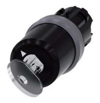
key-operated switch Siemens, 22 mm, round, plastic with metal front ring, special lock, with 2 keys, 2 switch positions O<I, momentary contact type, actuating angle  $45^\circ,\,10:\!30h/12h,$  key removal O
