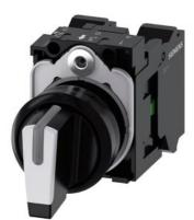
Selector switch, illuminable, 22 mm, round, plastic, white, selector switch, short, 3 switch positions I>O<II, momentary contact type, 10:30h/12h/13:30h, with holder, 1 NO, 1 NO, spring-type terminal, Z=20-unit packaging
