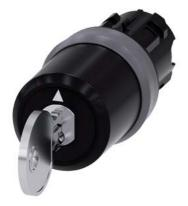
Key-operated switch BKS, 22 mm, round, plastic with metal front ring, lock No. E9 (VW), without key, 3 switch positions I-O-II, latching, actuating angle  $2x45^{\circ}$ , 10:30h/12h/13:30h, Key removal I+O+II, with laser labeling, upper case
