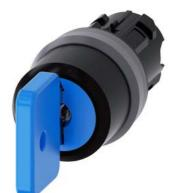
Key-operated switch O.M.R, 22 mm, round, plastic with metal front ring, lock number 73038, blue, with 2 keys, 3 switch positions I-O-II, latching, actuating angle 2x45°, 10:30h/12h/13:30h, Key removal I+O+II, with laser labeling, upper case
