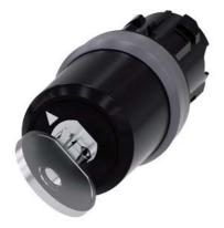
Key-operated switch BKS, 22 mm, round, plastic with metal front ring, lock number S1, with 2 keys, 2 switch positions O<I, momentary contact type, Actuating angle  $45^{\circ}$ , 10:30h/12h, Key removal O
