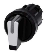
Selector switch, illuminable, 22 mm, round, plastic, white, selector switch, short, 3 switch positions I>O<II, momentary contact type, actuating angle 2x45°, 10:30h/12h/13:30h, with laser labeling, upper case
