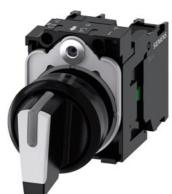
Selector switch, illuminable, 22 mm, round, plastic, white, selector switch, short, 3 switch positions I>O<II, momentary contact type, 10:30h/12h/13:30h, with holder, 1 NO, 1 NO, screw terminal
