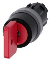
Key-operated switch O.M.R, 22 mm, round, plastic with metal front ring, lock number 73037, red, with 2 keys, 3 switch positions I>O<II, momentary contact type, actuating angle 2x45°, 10:30h/12h/13:30h, key removal O, with laser labeling, lower case
