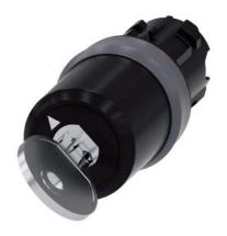
Key-operated switch BKS, 22 mm, round, plastic with metal front ring, Lock No. E7 (VW), without key, 2 switch positions O-I, latching, actuating angle 90°, 10:30h/13:30h, key removal O+I, with laser labeling, inscription or symbol Customer-specific selection with SIRIUS ACT configurator (CIN)
