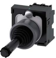
Coordinate switch, 22 mm, round, plastic with metal front ring, black, 2 switch positions, vertical, momentary contact type, with mechanical interlocking in O position, with holder, 1 NO, 1 NO, screw terminal
