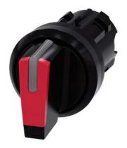
Selector switch, illuminable, 22 mm, round, plastic, red, selector switch, short, 3 switch positions I-O<II, left latching, right momentary contact type, actuating angle 2x45°, 10:30h/12h/13:30h, with laser labeling, upper case and lower case, always upper case at the beginning of the word
