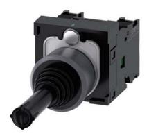
Coordinate switch, 22 mm, round, plastic with metal front ring, black, 2 switch positions, horizontal latching, without mechanical interlocking, in O position, with holder, 1 NO, 1 NO, screw terminal, with laser labeling, lower case
