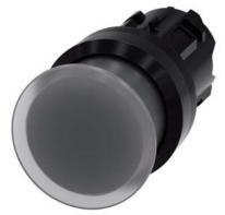
Illuminated mushroom pushbutton, 22 mm, round, plastic, clear, 30 mm, momentary contact type, with laser labeling, lower case  $\,$
