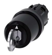
Key-operated switch IKON, 22 mm, round, plastic, lock number 360012K1, with 2 keys, 3 switch positions I-O-II, latching, actuating angle 2x45°, 10:30h/12h/13:30h, key removal O, with laser labeling, upper case and lower case, always upper case at the beginning of the word
