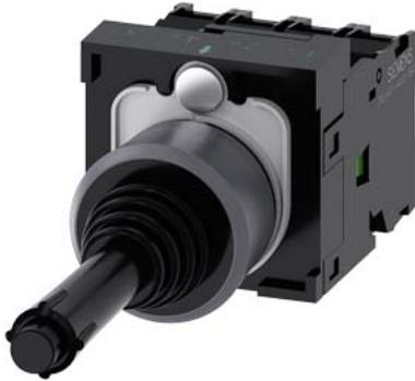
Coordinate switch, 22 mm, round, plastic with metal front ring, black, 4 switch positions, momentary contact type, with mechanical interlocking in O position, with holder, 1 NO, 1 NO, 1 NO, 1 NO, screw terminal, Z=20-unit packaging
