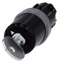
key-operated switch Siemens, 22 mm, round, plastic with metal front ring, lock number SSG10, with 2 keys, 2 switch positions O-I, latching, actuating angle  $90^\circ, 10:30h/13:30h,$  key removal I, with laser labeling, upper case and lower case, always upper case at beginning of line
