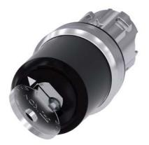
Key-operated switch IKON, 22 mm, round, metal, shiny, lock number 360012K1, with 2 keys, 2 switch positions O-I, latching, actuating angle  $90^\circ$ , 10:30h/13:30h, key removal O+I, with laser labeling, upper case
