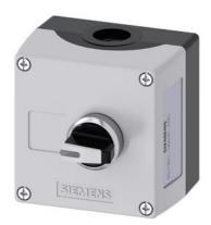
Enclosure for command devices 22 mm, round, enclosure material plastic, enclosure top part gray, 1 control point, A = Selector switch, black, metal, 3 switch positions, momentary contact type, 1 NO, 1 NO, spring-type terminal, floor mounting, support terminal, recess for label, 1xM20 each on top and bottom
