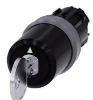
Key-operated switch BKS, 22 mm, round, plastic with metal front ring, lock number S1, with 2 keys, 3 switch positions I-O-II, latching, actuating angle 2x45°, 10:30h/12h/13:30h, Key removal I+II, with laser labeling, upper case
