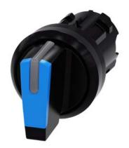
Selector switch, illuminable, 22 mm, round, plastic, blue, selector switch, short, 3 switch positions I>O<II, momentary contact on the left, latching on the right, actuating angle 2x45°, 10:30h/12h/13:30h, with laser labeling, upper case and lower case, always upper case at the beginning of the word
