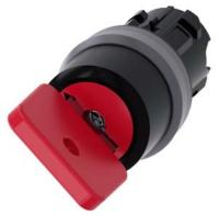
Key-operated switch O.M.R, 22 mm, round, plastic with metal front ring, lock number 73037, red, with 2 keys, 2 switch positions O<I, momentary contact type, Actuating angle 45°, 10:30h/12h, key removal O, with laser labeling, lower case
