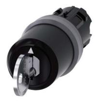
Key-operated switch IKON, 22 mm, round, plastic with metal front ring, lock number 360012K1, with 2 keys, 3 switch positions I-O-II, latching, actuating angle 2x45°, 10:30h/12h/13:30h, Key removal I+O+II, with laser labeling, lower case
