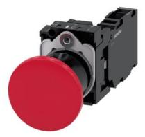
Mushroom pushbutton, 22 mm, round, plastic, red, 40mm, latching, pull-to-unlatch mechanism, with holder, 1 NO+1 NC, screw terminal, with laser labeling, upper case and lower case, always upper case at the beginning of the word
