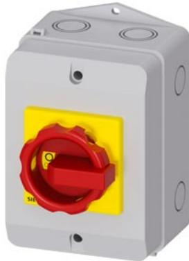
SETRON, Switch disconnecter 3LD, emergency switching-off switch, 3- pole, Iu: 16 A, operating power / at AC-23 A 400 V: 7.5 kW, Molded plastic encapsulation for inch cable gland, 1 NC, 1 NO, rotary operating mechanism, red/yellow
