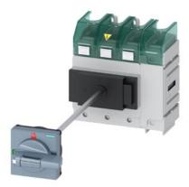
SENTRON, Molded case switch 3LD5 UL, Main switch, 4-pole, certified according to UL489 UL60947-4-1 and IEC60947-3, UL: 100A, SCCR 65kA at 480VAC, Operating power at 480VAC 3-phase: 60hp, IEC: 100A, Operating power at AC-23A at 400V: 45kW, floor mounting with door coupling rotary operating mechanism, defeatable, Standard, 4-hole mounting of the handle, without tolerance compensation, incl. terminal covers for the infeed side
