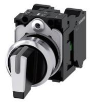
Selector switch, illuminable, 22 mm, round, metal, shiny, white, selector switch, short, 3 switch positions I-O-II, latching, actuating angle 2x45°, 10:30h/12h/13:30h, with holder, 1 NO, 1 NO, Spring-type terminal
