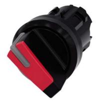
Selector switch, illuminable, 22 mm, round, plastic, red, selector switch, short, 2 switch positions O<I, momentary contact type, Actuating angle 45°, 10:30h/12h, with laser labeling, upper case
