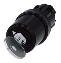
keyswitch BKS, 22 mm, round, plastic, special lock, with 2 keys, 2 switch positions O-I, latching, actuating angle 90°, 10:30h/13:30h, key removal O+I, note: for the BKS locking systems E1 - E25 supplied without key
