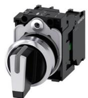
Selector switch, illuminable, 22 mm, round, metal, shiny, white, selector switch, short, 3 switch positions I>O<II, momentary contact type, actuating angle 2x45°, 10:30h/12h/13:30h, with holder, 1 NO, 1 NO, screw terminal, Z=20-unit packaging
