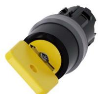
Key-operated switch O.M.R, 22 mm, round, plastic with metal front ring, lock number 73033, yellow, with 2 keys, 2 switch positions O-I, latching, actuating angle 90°, 10:30h/13:30h, key removal O, with laser labeling, upper case
