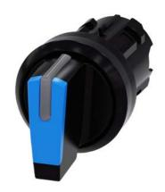
Selector switch, illuminable, 22 mm, round, plastic, blue, selector switch, short, 3 switch positions >O<II, momentary contact on the left, latching on the right, actuating angle  $2x45^\circ$ , 10:30h/12h/13:30h, with laser labeling, inscription or symbol Customer-specific selection with SIRIUS ACT configurator (CIN)
