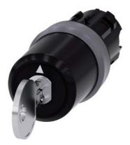
key-operated switch Siemens, 22 mm, round, plastic with metal front ring, lock number SSG10, with 2 keys, 3 switch positions I-O-II, latching, actuating angle 2x45°, 10:30h/12h/13:30h, key removal II, with laser labeling, lower case
