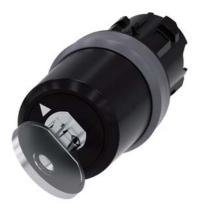
Key-operated switch BKS, 22 mm, round, plastic with metal front ring, lock number S1, with 2 keys, 2 switch positions O-I, latching, actuating angle  $90^\circ,$  10:30h/13:30h, key removal I, with laser labeling, inscription or symbol Customer-specific selection with SIRIUS ACT configurator (CIN)
