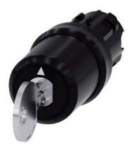
key-operated switch Siemens, 22 mm, round, plastic, special lock, with 2 keys, 3 switch positions I-O<II, left latching, momentary contact type on the right, actuating angle  $2x45^\circ,\,10:30h/12h/13:30h,\,key\,removal\,O+I$
