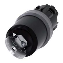
Key-operated switch IKON, 22 mm, round, plastic with metal front ring, lock number 360012K1, with 2 keys, 2 switch positions O-I, latching, actuating angle 90°, 10:30h/13:30h, key removal O, with laser labeling, upper case and lower case, always upper case at the beginning of the word
