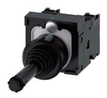
Coordinate switch, 22 mm, round, plastic, black, 2 switch positions, horizontal, momentary contact type, with mechanical interlocking in O position, with holder, 1 NO, 1 NO, screw terminal, with laser labeling, inscription or symbol Customerspecific selection with SIRIUS ACT configurator (CIN)
