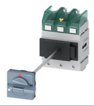
SENTRON, Molded case switch 3LD5 UL, Main switch, 3-pole, certified according to UL489 UL60947-4-1 and IEC60947-3, UL: 125A, SCCR 65kA at 480VAC, Operating power at 480VAC 3-phase: 75hp, IEC: 125A, Operating power at AC-23A at 400V: 55kW, floor mounting with door coupling rotary operating mechanism, defeatable, Standard, 4-hole mounting of the handle, without tolerance compensation, incl. terminal covers for the infeed side
