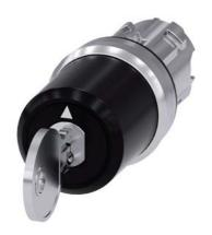
Key-operated switch BKS, 22 mm, round, metal, shiny, lock number S1, with 2 keys, 3 switch positions I-O<II, left latching, right momentary contact type, actuating angle 2x45°, 10:30h/12h/13:30h, key removal O, with laser labeling, upper case and lower case, always upper case at beginning of line
