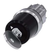
Key-operated switch BKS, 22 mm, round, metal, shiny, Lock number E1 (VW), without key, 2 switch positions O-I, latching, actuating angle 90°, 10:30h/13:30h, key removal O+I, with laser labeling, upper case and lower case, always upper case at the beginning of the word
