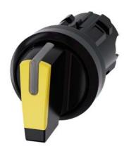
Selector switch, illuminable, 22 mm, round, plastic, yellow, selector switch, short, 3 switch positions I-O<II, left latching, right momentary contact type, actuating angle 2x45°, 10:30h/12h/13:30h, with laser labeling, upper case and lower case, always upper case at beginning of line
