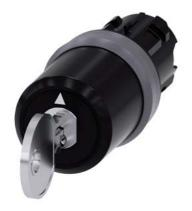
key-operated switch Siemens, 22 mm, round, plastic with metal front ring, lock number SSG10, with 2 keys, 3 switch positions I>O<II, momentary contact on the left, latching on the right, actuating angle  $2x45^{\circ}$ , 10:30h/12h/13:30h, key removal II Z=50-unit packaging
