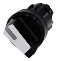
Selector switch, illuminable, 22 mm, round, plastic, white, selector switch, short, 2 switch positions O<I, momentary contact type, Actuating angle 45°, 10:30h/12h, with laser labeling, lower case
