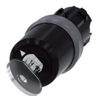
Key-operated switch BKS, 22 mm, round, plastic with metal front ring, Lock number E1 (VW), without key, 2 switch positions O-I, latching, actuating angle 90°, 10:30h/13:30h, key removal O+I, with laser labeling, inscription or symbol Customer-specific selection with SIRIUS ACT configurator (CIN)
