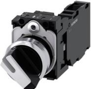
Selector switch, illuminable, 22 mm, round, metal, shiny, white, selector switch, short, 2 switch positions O-I, latching, actuating angle  $90^{\circ}$ , 10:30h/13:30h, with holder, 1 NO+1 NC, screw terminal
