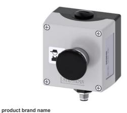
Enclosure for command devices, 22 mm, round, enclosure material metal, enclosure top part gray, 1 control point metal, A=Mushroom pushbutton, black, 40 mm, momentary contact type, 1 NO, spring-loaded terminal, floor mounting, silver label, black font, with graphic symbol: Autoplay, M12 connector (5-pin) bottom, insulated reserve conductors Label glued in
