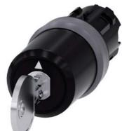
Key-operated switch BKS, 22 mm, round, plastic with metal front ring, lock number S1, with 2 keys, 3 switch positions I>O<II, momentary contact on the left, latching on the right, actuating angle 2x45°, 10:30h/12h/13:30h, key removal O, with laser labeling, Customer-specific selection with SIRIUS ACT configurator (CIN)
